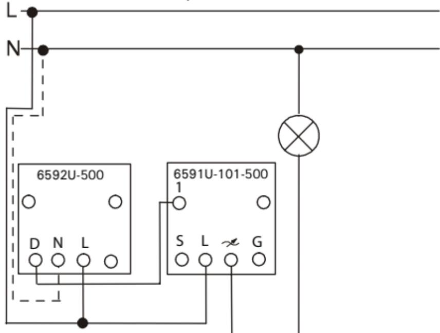
5 extension units maximum can be operated in parallel.
